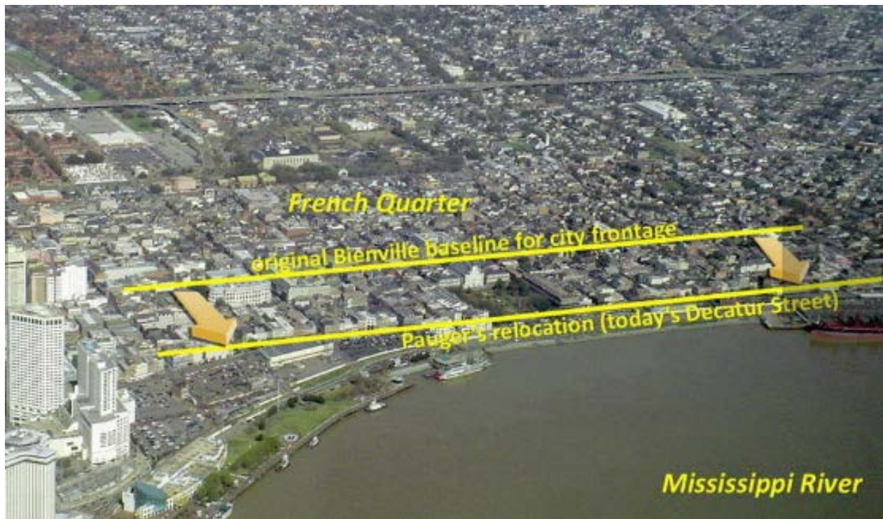
Assistant engineer Adrien de Pauger, arrived at New Orleans in March 1721, soon came to realize that Bienville's original baseline, set so far back from the river, needlessly squandered valuable high ground, and proposed to move it to today's Decatur Street. Graphic by Richard Campanella.
