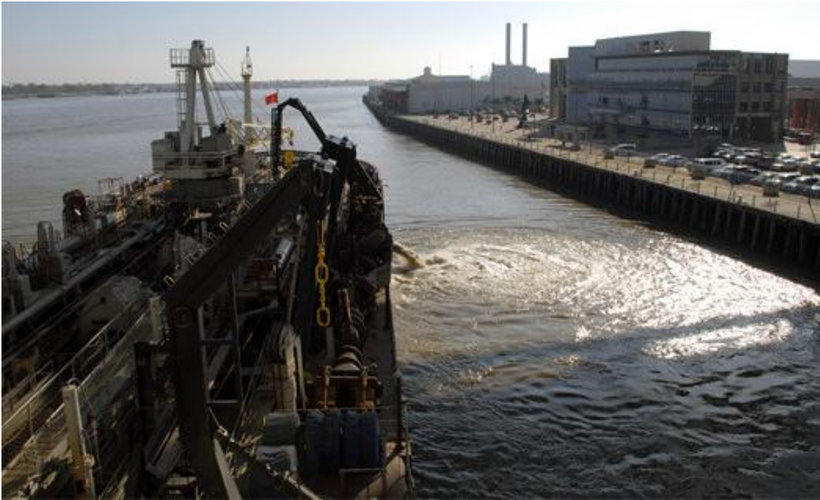
Hopper dredge, New Orleans Harbor. [Photo by Ricky Boyett, courtesy of the USACE]
