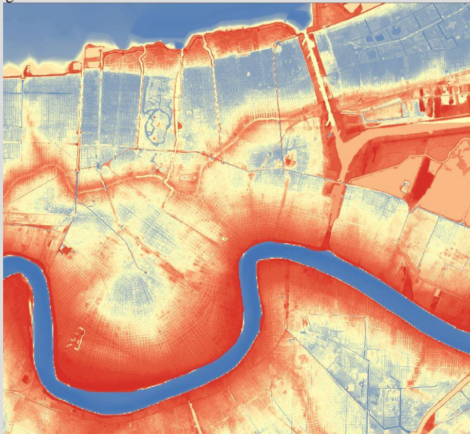
LIDAR elevation model of New Orleans, showing areas above sea level in red tones and below sea level in yellow-to-blueish tones_Graphic by Richard Campanella
