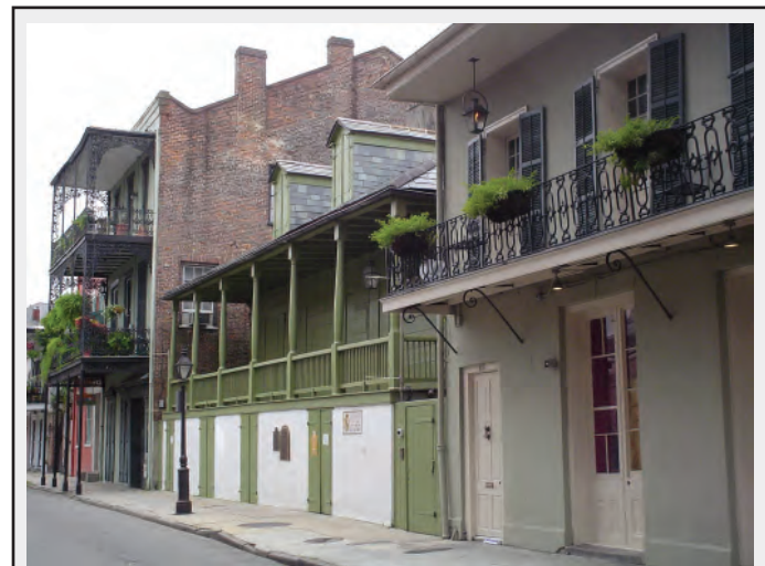
This Dumaine streetscene presents three ways in which New Orleanians have buffered the private space of the house with the public space of the street: with a narrow balcony (early nineteenth century, foreground); with a spacious wooden gallery under an oversized roof (center, late eighteenth century), and with a three-story cast-iron gallery as wide as the sidewalk (mid-nineteenth century). Photograph by author, 2004.
